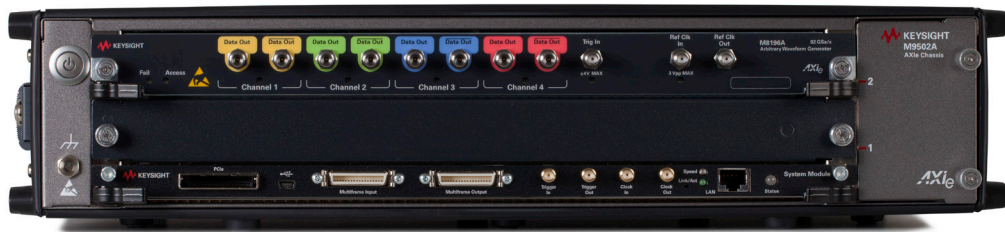
M8196A in a 2-slot AXIe chassis
